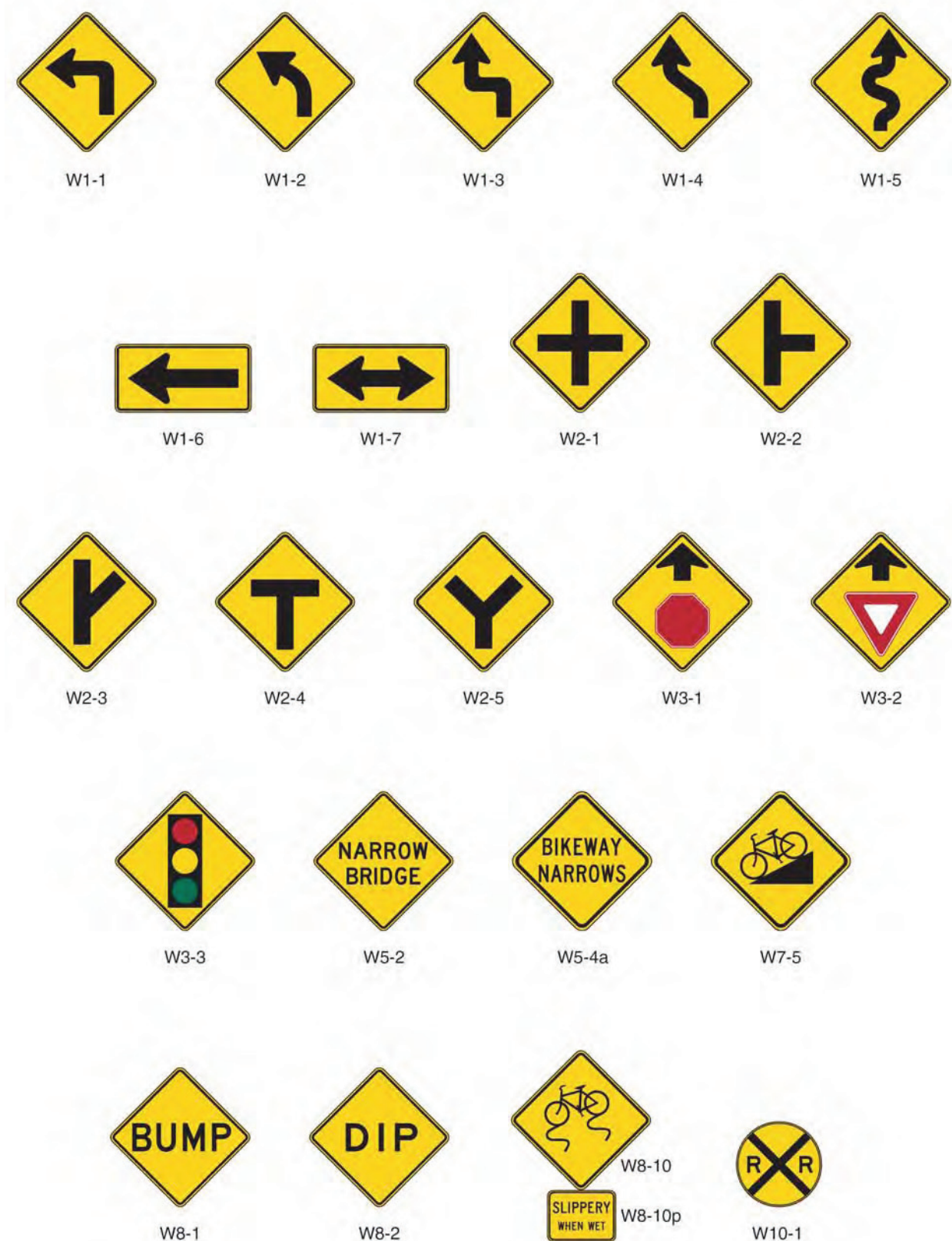
Figure 9B-3. Warning Signs for Bicycle Facilities (Sheet 1 of 2)
