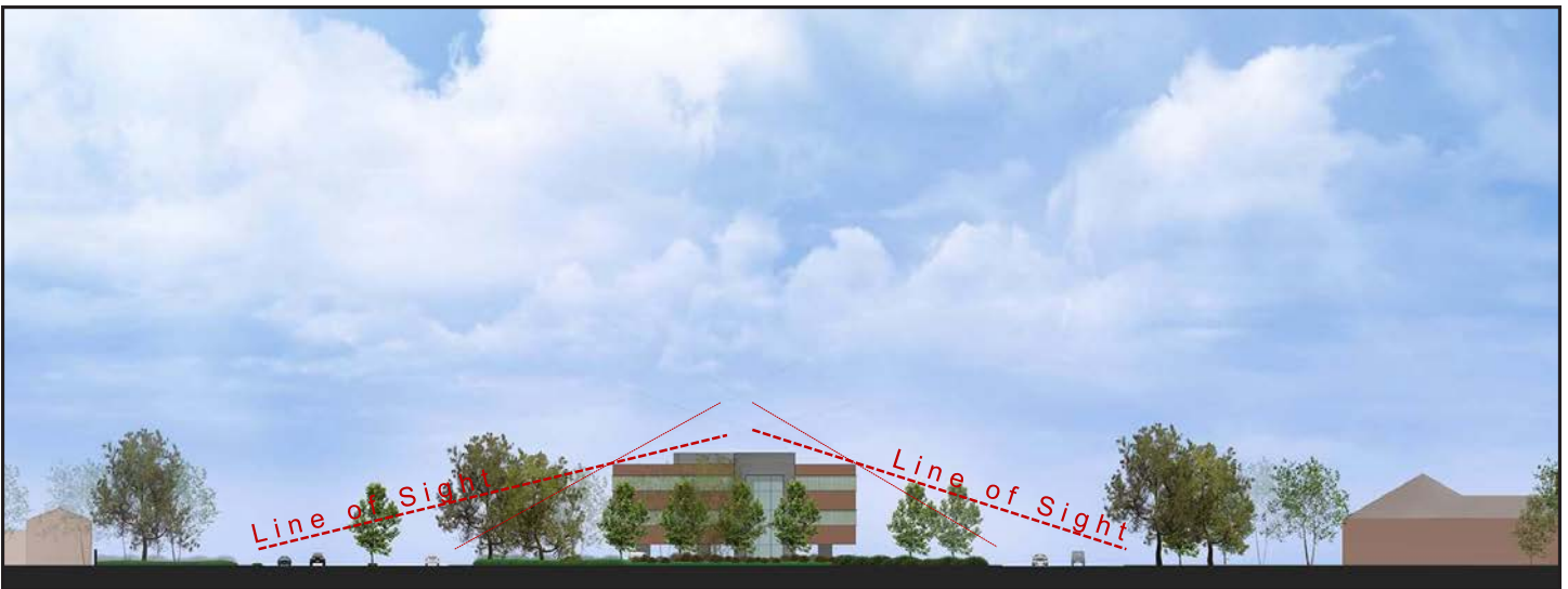
West Elevation - Lines of Sight drawn from pedestrian eye level on all four sidewalk locations.
